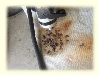
Next, remove every rubber fuel line, then use a compressor and an air nozzle to blow through the metal line that runs to the engine. Wrap a clean rag around the end of the line so you can see what's coming out. If it's rusty, continue to blow until it's not. Replace with new rubber fuel lines.
